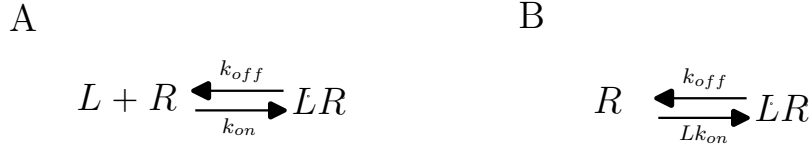
Figure 3: Dissociation-association models. Classic models about interaction between ligand and receptors when the ligand is considered as a constant (B) or not (A).
